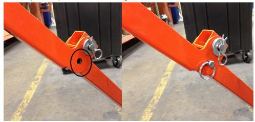
3. Once the handle is open, unfold the lifting arm. You will experience some slight resistance when unfolding. This is to help ensure the lift arm does not collapse on your fingers when the lift is folded back up.
