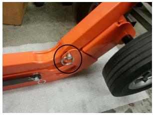
2. Unfold top handle and insert the quick release pin through the bracket and tube to lock the handle in place as show below. Make sure pin is fully inserted before using the lift.
