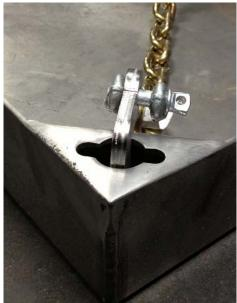
2. Once the hooks are in place feed the chain through the lift box until the chain is pulled tight in all four directions.
