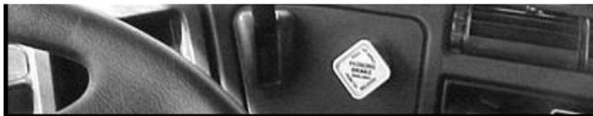
**Figure 3.** The *Copilot*® was mounted on the truck dash for measurement of slow eyelid closures (PERCLOS) during driving. (See Appendix A-1 for additional photos of the *Copilot*®, and Appendix B-1 on instructions to drivers regarding )
