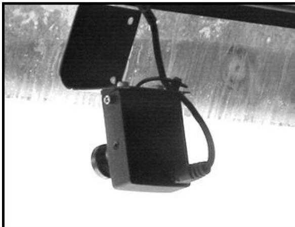
**Figure 4.** *SafeTRAC*® lane-tracking monitor developed by AssistWare Technology. *SafeTRAC*® employs a video camera mounted on the truck windshield (or truck podium) and coupled to a small computer that continuously analyzes the road, lane markings, and other roadway features. (See Appendix A-1 for additional photos of *SafeTRAC*®, and Appendix B-1 for instructions to drivers regarding *SafeTRAC*®.)
